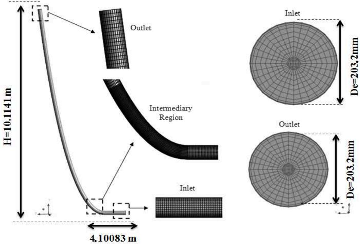
Figure 1. Geometrical parameters of the riser.
