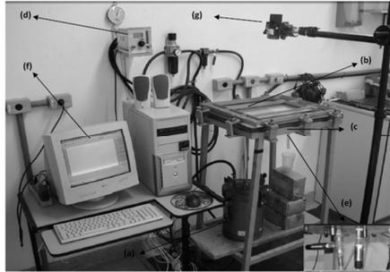
Fig. 1 - Photo of the RTM experimental apparatus from LACOMP/UFRGS: (a) pressure vessel, (b) strengthened glass top mold, (c) steel lower mold, (d) pressure controller, (e) pressure transducers, (f) data acquisition system and (g) camera.
