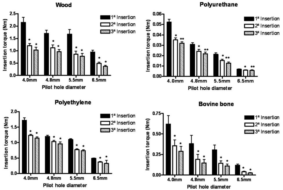
Figure 4. Histograms illustrating the insertion torque of 7-mm screws inserted into pilot holes of different diameters. The asterisk (\*) indicates a statistically significant difference to values of the first insertion into the specific diameters of the pilot hole. \*\* Indicates significant difference to values of first and second insertion into the specific diameters of the pilot hole.
