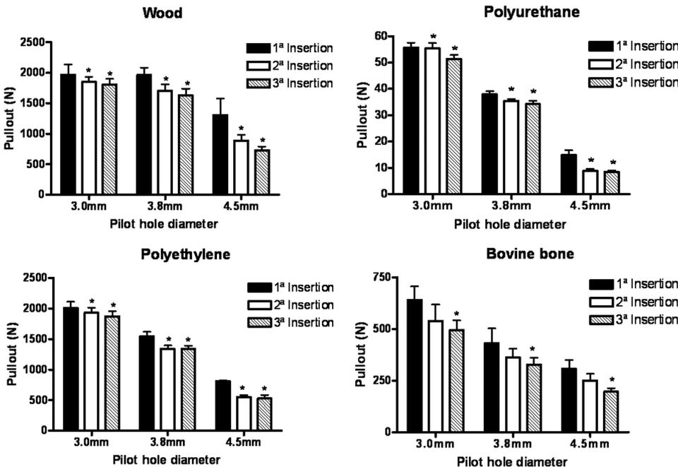
Figure 5. Histograms illustrating the pullout strength of 5-mm screws inserted into pilot holes of different diameters and different materials. The asterisk (\*) indicates a statistically significant difference to values of the first insertion into the specific diameters of the pilot hole. \*\* Indicates significant difference to values of first and second insertion into the specific diameters of the pilot hole.
