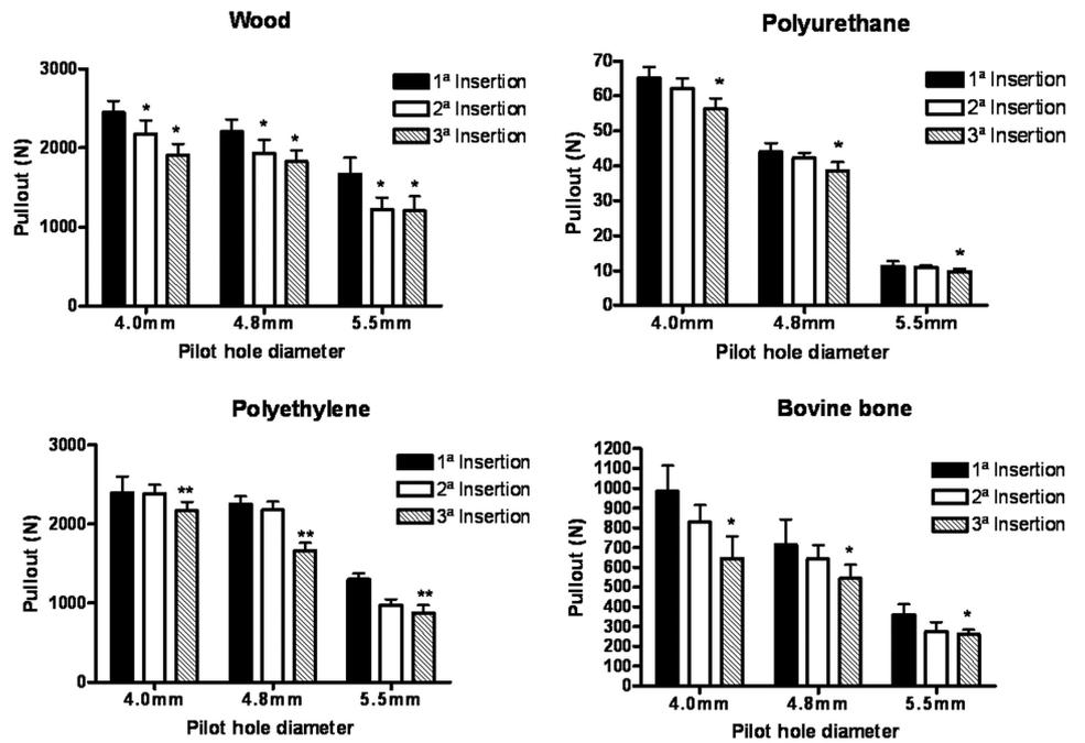
Figure 6. Histograms illustrating the pullout strength of 6-mm screws inserted into pilot holes of different diameters in different materials. The asterisk (\*) indicates a statistically significant difference to values of the first insertion into the specific diameters of the pilot hole. \*\* Indicates significant difference to values of first and second insertion into the specific diameters of the pilot hole.
