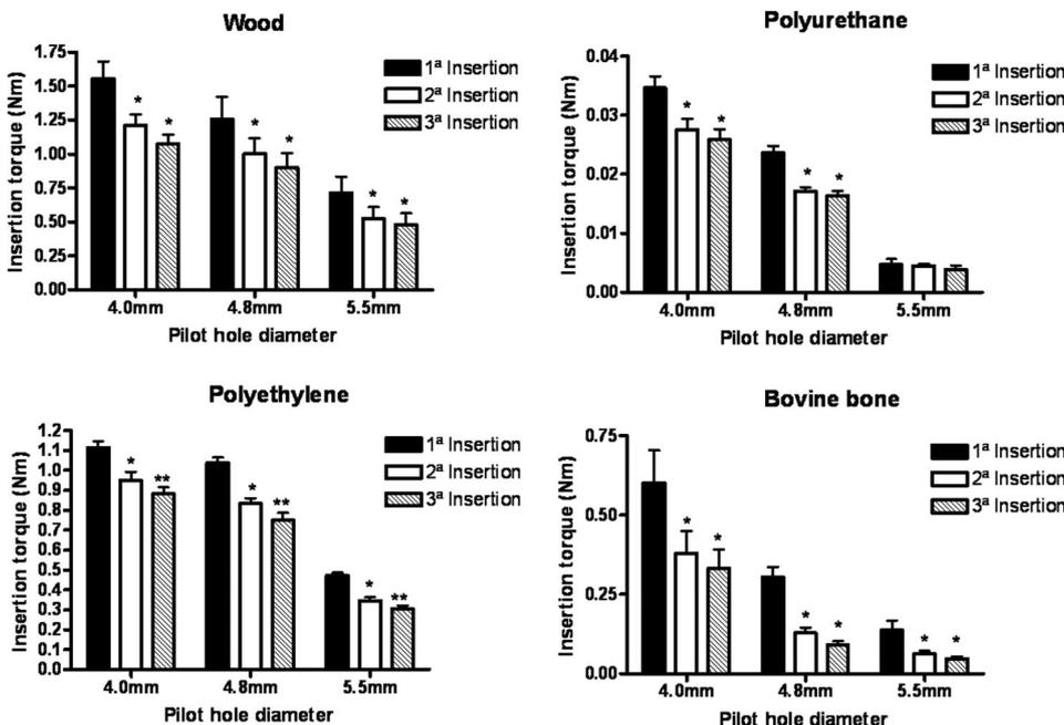
Figure 3. Histograms illustrating the insertion torque of 6-mm screws driven into pilot holes of different diameters. The asterisk (\*) indicates a statistically significant difference to values of the first insertion into the specific diameters of the pilot hole. \*\* Indicates significant difference to values of first and second insertion into the specific diameters of the pilot hole.
