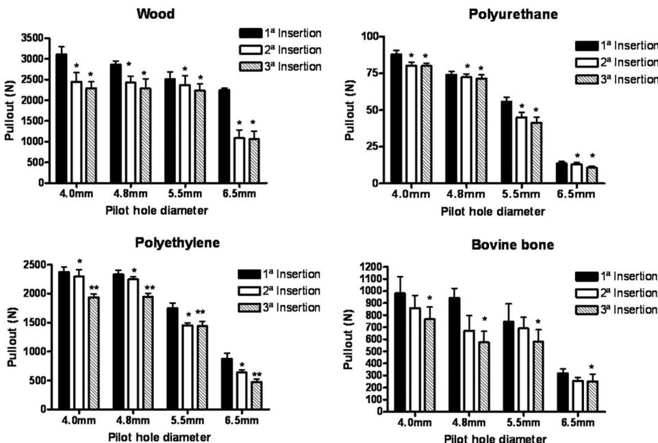
Figure 7. Histograms illustrating the pullout strength of 7-mm screws inserted into pilot holes of different diameters in different materials. The asterisk (\*) indicates a statistically significant difference to values of the first insertion into the specific diameters of the pilot hole. \*\* Indicates significant difference to values of first and second insertions into the specific diameters of the pilot hole.
