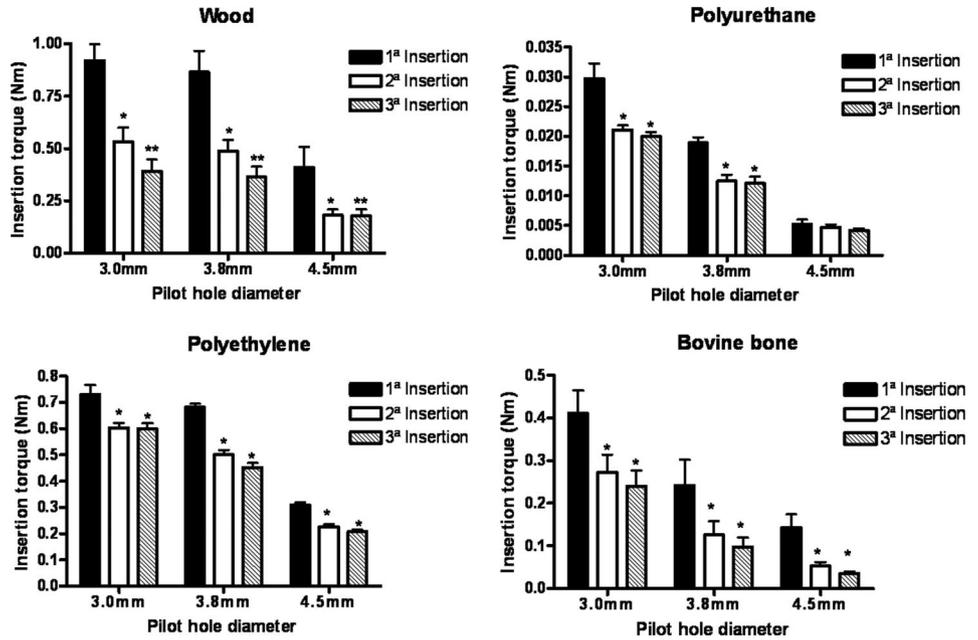
Figure 2. Histograms of the insertion torque of 5-mm screws driven into pilot holes of different diameters. The asterisk (\*) indicates a statistically significant difference to values of the first insertion into the specific diameters of the pilot hole. \*\* Indicates significant difference to values of first and second insertion into the specific diameters of the pilot hole.
