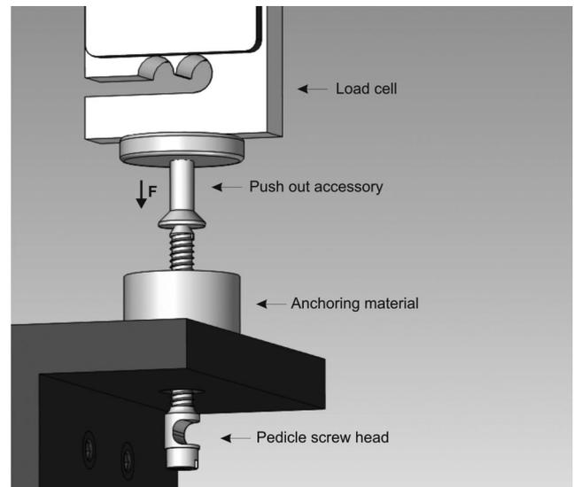
Figure 1. Schematic of the pushing out test. The block was placed on a support with the tip of the screw protruding 1 cm and pointing upward. A metal accessory protected the screw tip and provided an adequate surface for load application.
